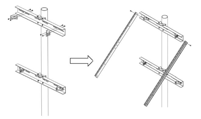
Attach panel rails to upper saddle L-brackets using 5/16" hardware provided. Apply anti-seize.
