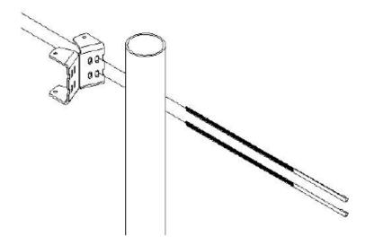
When using band clamps, tighten to 4-5 ft-lb torque. Wiggle saddle bracket to remove slack in band clamps and retighten. Repeat until clamps are snug.
