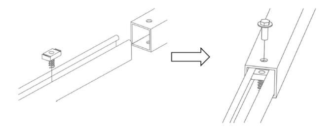
OPTIONAL: Drop spring nut into tilt leg strut and rotate to lock into place. Slide strut and spring nut into tilt leg tube and adjust to desired length. Longer legs, decrease tilt: shorter legs, increase tilt. Tighten 3/8" hardware using 9/16" wrench to 18-20 ft-lb torque.
