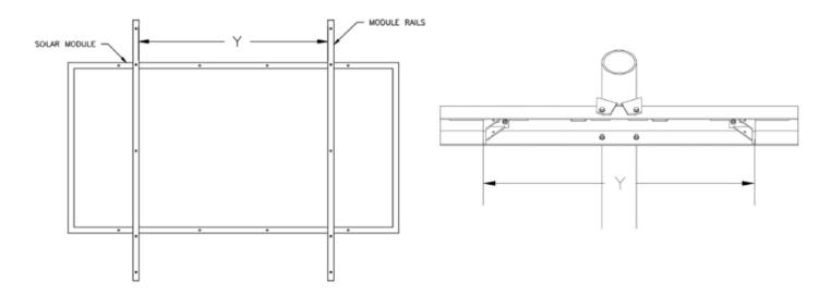
Lay rails on module holes (but do NOT attach) to determine angle bracket spacing (see image below). Measure between the inside of the module rails. Mount angle brackets to saddles using the 5/16" hardware provided. Tighten using 1/2" wrench to 10-12 ft-lb torque. Apply anti-seize.
