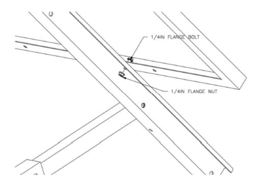
Mount the solar modules to the rails using the 1/4" hardware provided.
