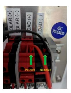
After the Master Edge is securely mounted to the enclosure, connect the load wire to the Master Edge power input.
