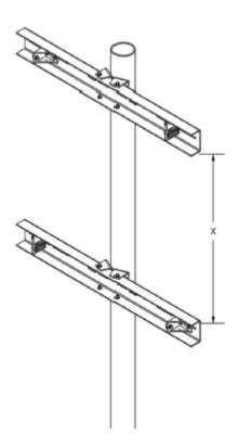
Loosely fasten the lower easy mount bracket to the pole. Use the below chart for rough spacing between the two saddles.
