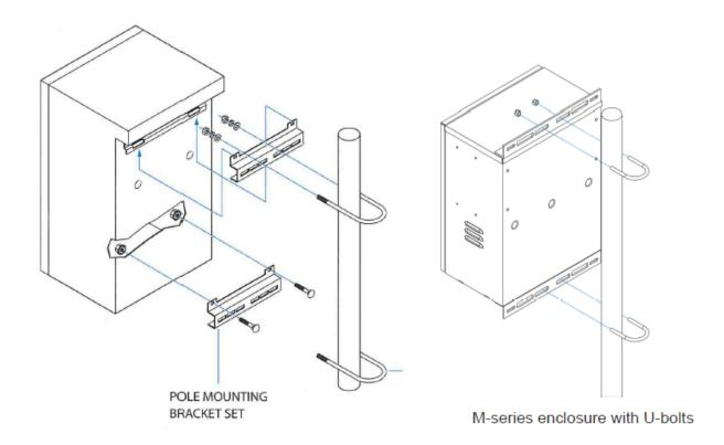
1. Mount the upper mounting bracket at the desired height of the enclosure on the pole using U-bolts.
