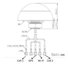
These adapters are screwed in on the GPS, Cell 1 and Cell 2 SMA terminals on the Master Edge, leaving only the WiFi connector without any adapter.
