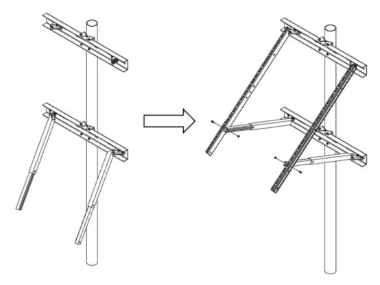
Attach tilt legs to lower saddle L-brackets. Adjust the tilt angle by adjusting the tilt arms and lower saddle to the desired angle of tilt then tighten the U-bolt/band clamp on the lower saddle. For 5/16" hardware tighten using 1/2" wrench to 10-12 ft-lb torque.
