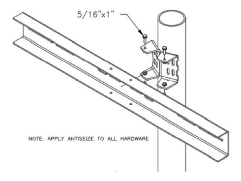
Fasten the saddle bracket to the easy mount bracket using the provided 5/16"" hardware. For 5/16" hardware, tighten using a 1/2" wrench to 10-12 ft-lb torque. Apply anti-seize.
