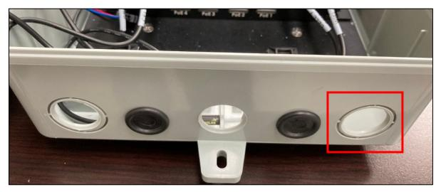
Figure 3: Grommet Location on Enclosure
