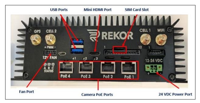
Figure 4: Device Connections
